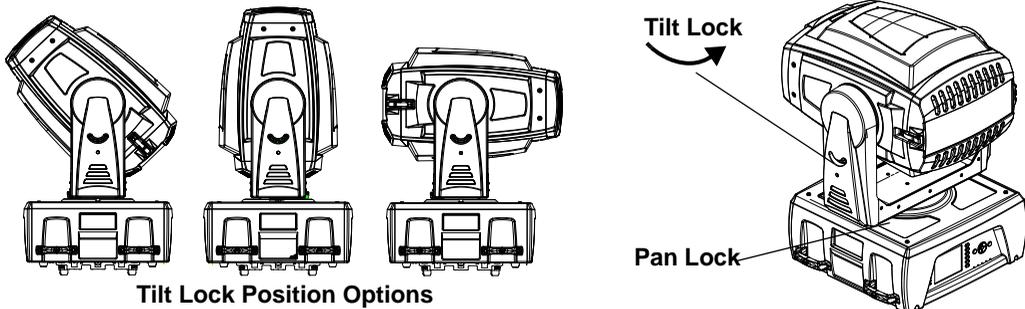
**NOTE:** *Disengage Pan and Tilt locks before operating the fixture.*
