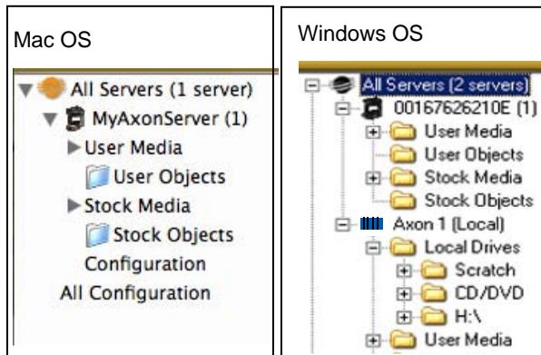
**NOTE:** *Tree structure differs slightly on the two platform versions. In the Mac version, to access Server Configuration information for an individual server, select the Configuration option under the individual server. In Windows Explorer, configuration information for the server is located directly by selecting the server.*
