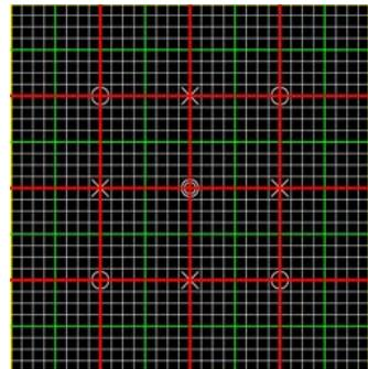
**TIP:** Before you begin other adjustments, physically view the grid from along the centerline of the fixture. The centerline of the grid should align with the center of the sphere. You can easily adjust any variation using the Pan channel. The object is to align the vertical lines of the guide with the vertical axis of the sphere.
