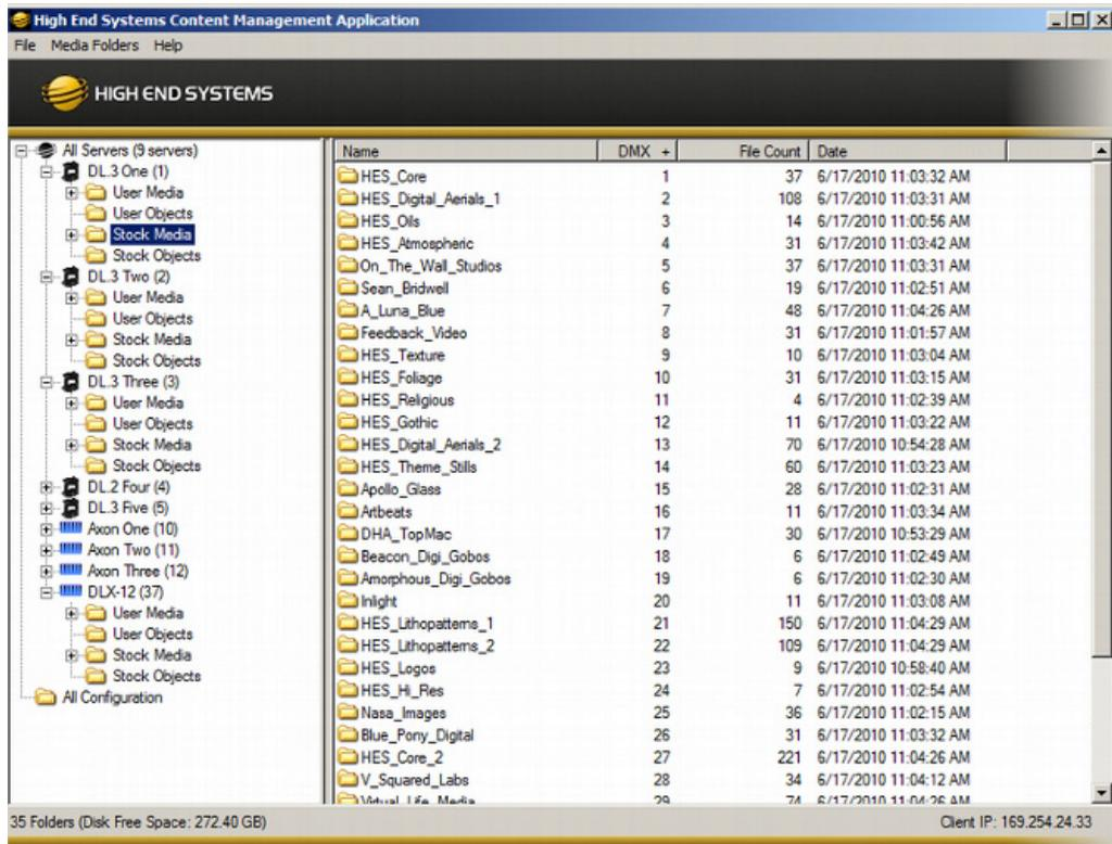
A **Status Bar** at the bottom of the page, indicates the number of files or folders in a selected folder in the left pane, as well as free space on the local computer hard drive and its IP address.
