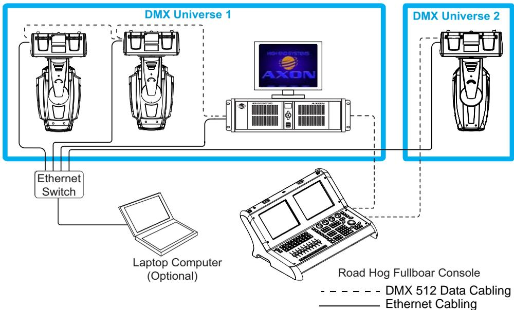
**NOTE:** *If you are using a DMX console and other automated lighting products compatible with Art-Net, this network can also serve as the link for DMX control.*
