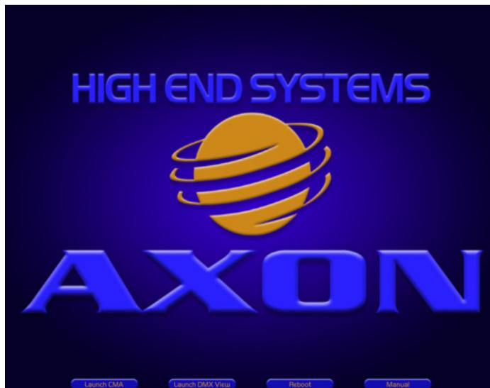
**NOTE:** *An active display device must be attached to both DVI ports before booting up the system. When only one port is connected, it defaults to display the graphics engine output and will not display the CMA screen.*
