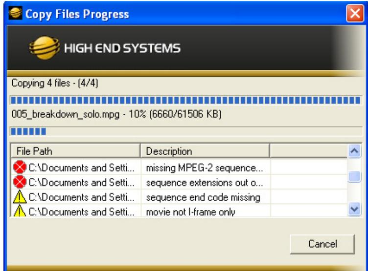
**NOTE:** Since the CMA executes the scanning/copying process for the entire group of folders/files in a single operation, it will not stop or pause during the process to dismiss the errors.
