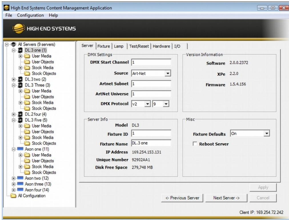
2. Select a **DMX Source** type by clicking on the down arrow of the Source field to select DMX512 or Art-Net.
