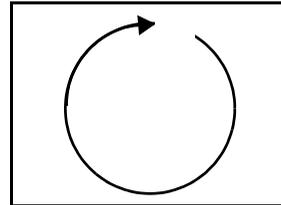
The Rotation parameters' suggested default values are the midpoint of the 16-bit DMX value range, which is equal to no rotation. Increasing the DMX value from the midpoint indexes the object in a clockwise direction. Reducing the DMX value below the midpoint indexes the object in a counterclockwise direction.
