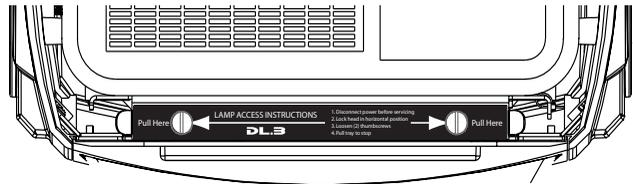
7. Loosen the thumbscrew and open the lamp cover.
