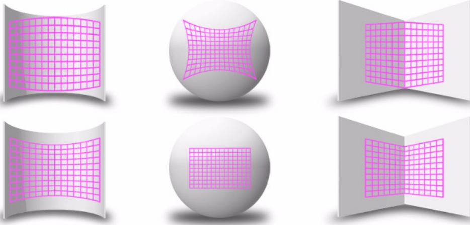
You can apply this correction to any media server output including multi-fixture image panoramas created with the Collage Generator Effect, (see *Global Functions: Collage Generator™ Effect* on page 135).
