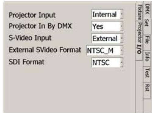
**Projector In By DMX** toggles the ability to set the projector input via the Control Console. **Yes** is the default and allows the input to be changed via the console, **No** doesn't allow the input to be changed.
