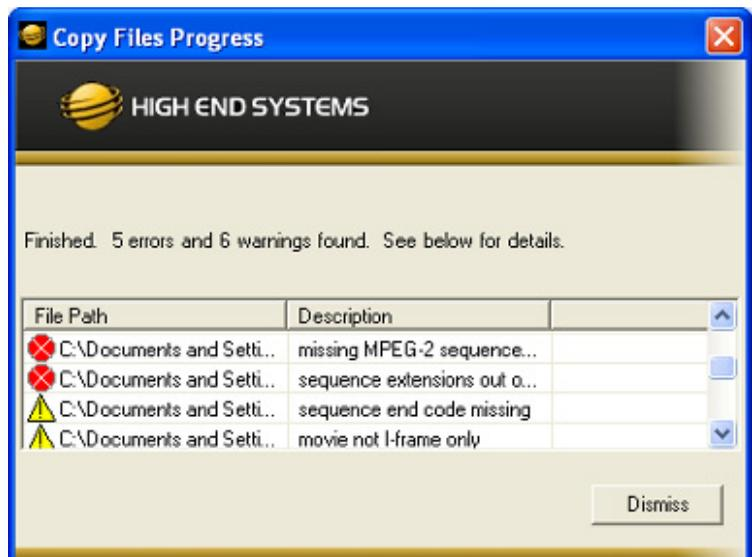
The files with errors in a group of files will not be copied on to the server. Files with warnings will be copied. They will show up highlighted in yellow when viewed in the “Details” view in the CMA to indicate to the user that this file is problematic.
