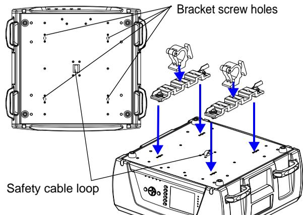
3. Run the safety cable through the loop on the fixture's base, and around the truss.
