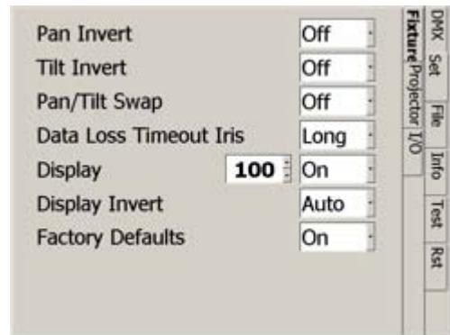
Setting the **Tilt Invert** field to **On** inverts the direction of the tilt motor. Use this option to coordinate movements between fixtures facing each other in a vertical orientation. **Off** is the default setting.
