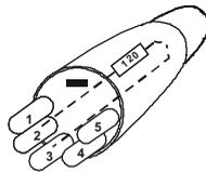
**Terminator:** 5-pin male XLR connector with a 120 Ohm terminating resistor fitted between pins 2 and 3.
