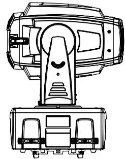
6. Loosen the two thumbscrews holding the projector bracket and slide the projector out of the fixture.
