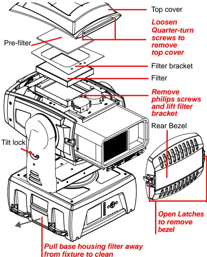
7. Remove the bracket and remove the HEPA filter from filter housing. Inspect both the prefilter and the HEPA filter.
