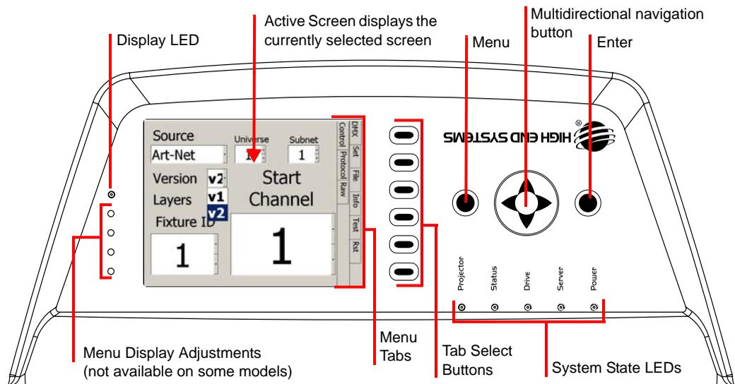
The LCD screen displays the menu system arranged with a series of **Menu Tabs** along the side for accessing configuration screens and options on the currently active screen. Clicking on one of the **Tab Select** buttons selects the screen tab next to it.
